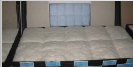
Figure 4.2: "Oliy and "Yahshi" cotton samples are naturally white and have a low trash content. (V. Gurney)
